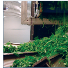
An example of a custom-built Bilwinco distribution tool for pre-cut lettuce leaves. The internal surface of the tool is optimised for lettuce
