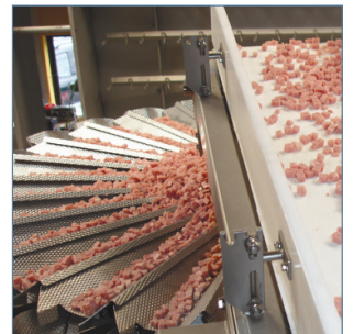
The conveyor loading the Linear Drive radial feeders
