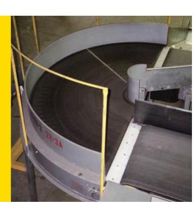
A compact, quiet and reliable 180 degree belt power curve.
