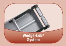
What is it? The conveyor headplates, which retain the conveyor pulleys and belt tension racks, are slightly tapered.
