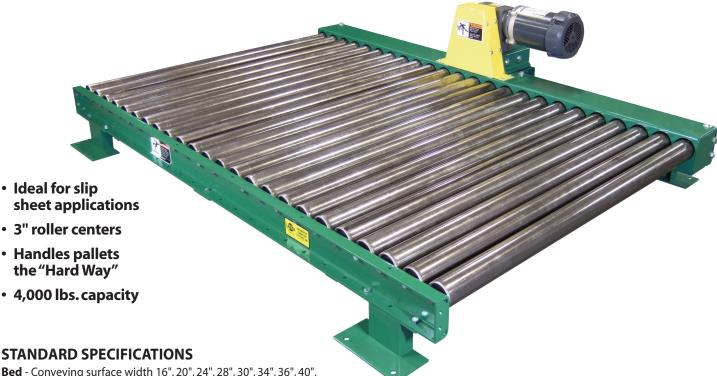
**Bed** - Conveying surface width 16", 20", 24", 28", 30", 34", 36", 40", 44", 48", 52", and 56". Heavy duty 4" and  $4^{3}/_{4}$ " deep x 4 gauge powder painted formed steel channel frame with heavy duty cross braces. Frames are bolted together with butt couplings and floor supports.
